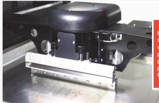
Independent, dual squeegee print head with programmable printing speeds and pressure for quality printing results each time
